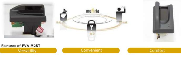
"FVA-M2ST" has versatility to various system devices as finger vein patterns used for authentication will be encrypted and stored outside module.
